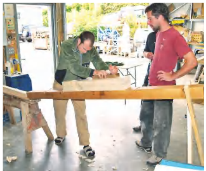
▲ Pic.12 A Japanese planing beam. This timber needed a couple of strokes with a finely-set plane to get it to fit
